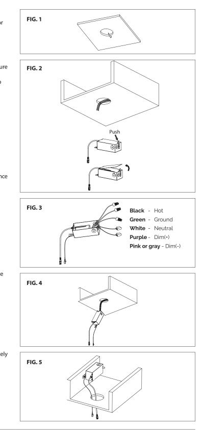
5. Guide junction box through the cut hole and secure appropriately using the external key hole (See **FIG. 5**).
